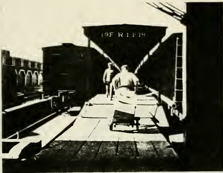
FIG. 72.—Loading goods at New York into railway cars on car-transfer floats for transport across the Hudson River.
